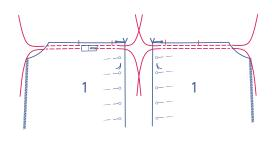
Starting just past the indicated notch, sew 2 parallel rows of stitching at the top of the front using a long stitch length at a low thread tension. Take care not to catch the facing (the folded part)
