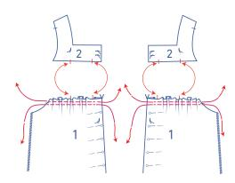
Distribute the ruffles so that the notches in the front match the notches in the top front (2).
