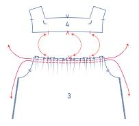
Distribute the ruffles so that the notches in the back match the notches in the top back (4).
