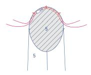
Sew two parallel rows of stitching from the top of the sleeve, using a long stitch length at a low thread tension. Sew just past the indicated single notches. Leave a length of thread at the start and end of the rows.
