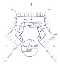
Snip diagonally towards the corners in the seam allowance. Note: to make clean right angles, snip until just before the marking thread!
