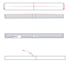
Fold the belt in half lengthwise with the right sides of the fabric facing.
