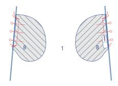
Pin the straight end of 2 of the 4 pocket pieces to the front, matching the marking threads. Sew into place between the marking threads.
