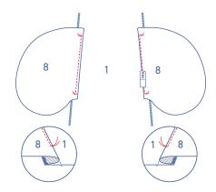
Fold the pocket and seam allowance over and sew the pocket to the seam allowance underneath.
