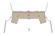
Pin and sew the back to the top back with the corresponding notches matching.
