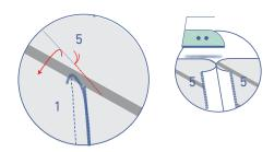
Now pin and stitch the short edge of the facing underneath the marking thread. Press the seam allowance open.
