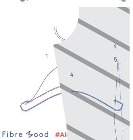
Fold the facing over and stitch to the seam allowance underneath from one marking thread to the other, right next to the seam.
