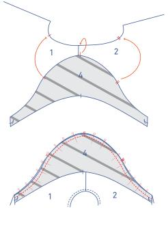
Pin and sew the top of the sleeve (= sleeve cap) (4) to the armhole, matching the notches. The single notch marks the front, while the double notch marks the back. The single notch at the top aligns with the shoulder seam.
