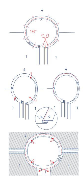
Sew the bias tape into place at 1/6" from the neckline. Snip off any excess bias tape (the exact length is not provided because the grainline is on the bias, i.e. it will differ according to fabric type).
