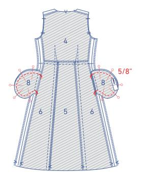
Pin and sew the contours of the pocket pieces together at 5%" from the raw edges.
