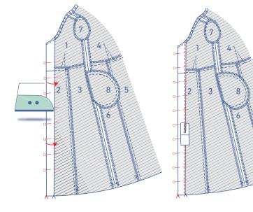
Neatly press the facing of the CF towards the wrong side at the indicated V notch at the bottom and pin into place.
