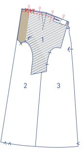
Pin and sew the bodice and skirt fronts together, matching the markings. The darts on the bodice and seams of the skirt should match.
