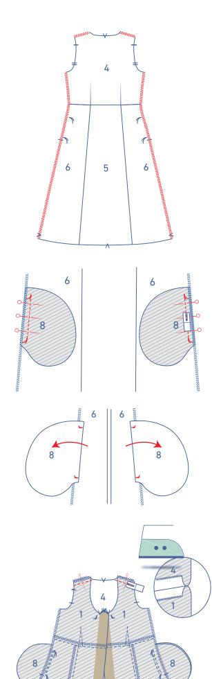
Finish the raw edges of the back where indicated with overlock stitching.
