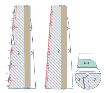
Pin and sew the seams of the skirt front (2) and skirt front side (3) pieces together, matching the markings.
