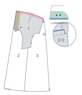
Finish the raw edges with overlock stitching. Press the seam allowance towards the front.
