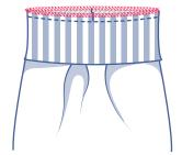
Finish the raw edges together with overlock stitching.
