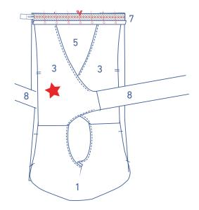
Pin and sew the top of the facing (unpressed edge) to the top of the CB piece (+ top piece back) as shown.
