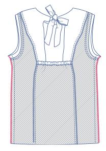
Finish the raw edges together with overlock stitching.
