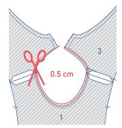
Trim the seam allowance on the neckline down by 0.5cm. This reduces bulk and allow the curves to lie flatter.
