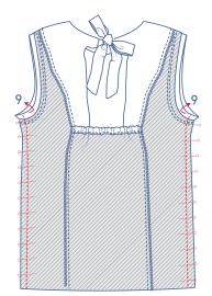
Pin and sew the side seams together (with the bias tape folded up).
