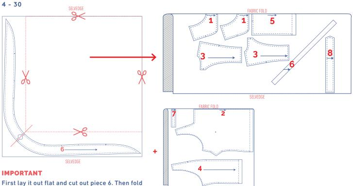
First lay it out flat and cut out piece 6. Then fold in half and cut the remaining pieces as shown.
