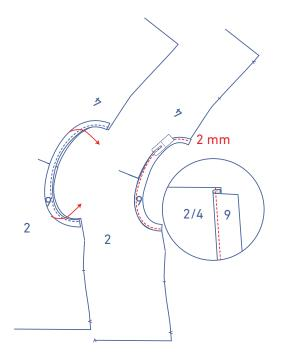
Fold the bias tape over and sew the bias tape through all layers right next to the seam (tape + seam allowance).
