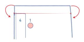
Fold the shaped facing down at the fold line on the top of the LF so that the right sides of the fabric are touching.
