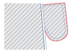
Finish the raw edges together with overlock stitching. Press the seam allowance of the side seams open.
