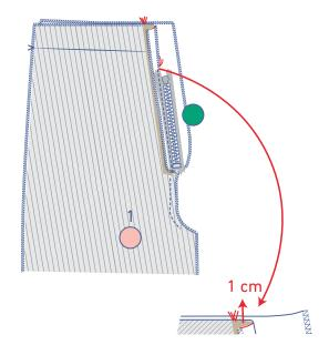
Close the zip and fold both front pieces so the right sides face each other. Ensure the V notches indicating the CF match. Smooth both pieces flat and pin the zip tape (marked with a red star) in place to the shaped RF fly (green dot).
