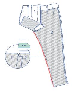
Finish the raw edges together with overlock stitching. Press the seam allowance towards the back.
