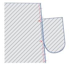
Pin the side seams. Sew from the top down to the marking thread at the top of the pocket opening. Now, sew from the next marking thread at the bottom of the pocket opening down to the hem.
