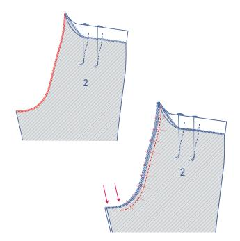
Fold the facing up at the CB and finish the CB seams separately with overlock stitching.
