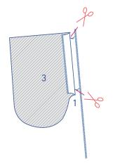
Fold back the seam allowance of the pocket at the front and snip diagonally into the front just up to the marking thread.
