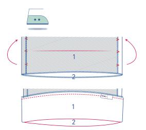
Fold over the hem to the centre-most V notches and sew into place right next to the overlocked edge.
