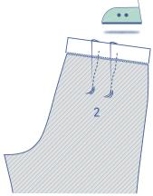
Turn the piece the wrong way out so that the wrong side of the back is facing up. Press the pleat allowance in the direction of the CB.
