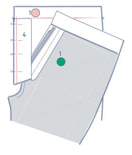
Line up the overlocked raw edges of the fly with the seam allowance of the LF and the zip. The finished top of the fly should be level with the fold line of the waistline's shaped facing. Pin and sew the fly to LF, going through all the layers (fly, zip, and LF).
