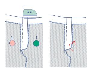
Press the fly to the side and close the zip. Sew the bottom of the shaped RF fly and the LF fly together with just a few stitches.
