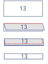
Fold the sleeve ties in (13) half lengthwise with the right side facing inwards. Sew the indicated edges closed.
