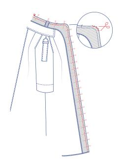
Pin and sew the CF and neckline of the garment and the facing into place all the way around. Trim the seam allowances and turn the facing onto the wrong side of the garment. Clip into the corners and trim, before pushing all the way out. Press flat.
