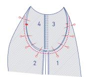
Pin and sew the armhole of the sleeve to the garment with the notches neatly aligned.
