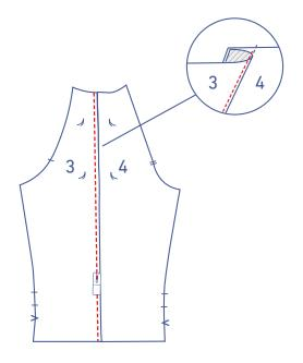
Press the seam allowance towards the sleeve front. Top stitch the sleeve front at 1/8" from the seam.
