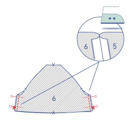
Pin and sew the side seams of the rain flaps. Press open the seam allowances.
