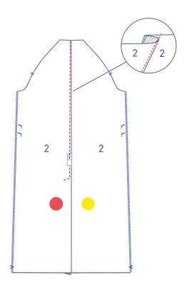
Top stitch the LB at 1/8" from the CB seam. Now pivot your needle and stitch the slanted edges at the top of the slit together too.
