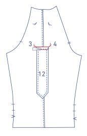
Pin the shoulder lapel fold to the top of the sleeve at the place indicated. The tip of the shoulder lapel should face the bottom of the sleeve. Sew into place at presser foot width.
